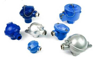
Terminal block located in a "head" allow for the connection of extension wires. Various materials are used for screw or solder terminations including copper, plated brass and, for the best performance in the case of thermocouples, thermoelement alloys. The various head styles cater for a wide variety of probe diameters and cable entries.
