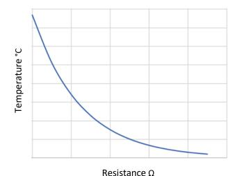
NTC thermistors are non-linear resistors that alter their resistance characteristics with temperature. Simply put, as temperature increases the thermistor's resistance decreases.
