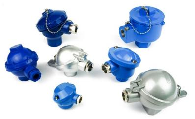
Terminal block located in a "head" allow for the connection of extension wires. Various materials are used for screw or solder terminations including copper, plated brass and, for the best performance in the case of thermocouples, thermoelement alloys. The various head styles cater for a wide variety of probe diameters and cable entries.
